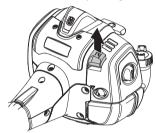
Remove the air filter cover and take out the filter. Blow clean with compressed air.
